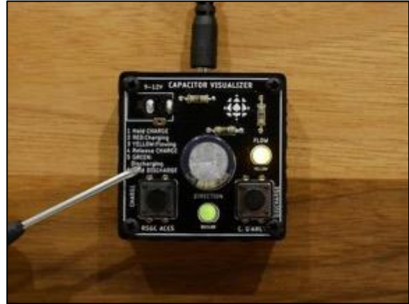
The capacitor acts like a battery and drains its charge through the green LED (PCB)
