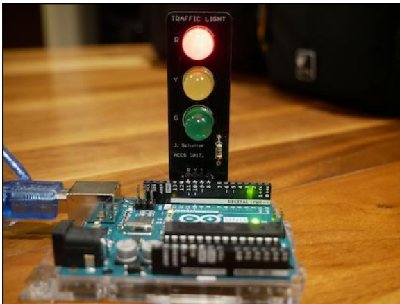
The Schaffer Traffic Light PCB in effect with the Arduino UNO
