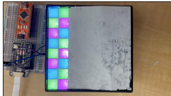
Lighting up some pixels of the small RGB matrix
