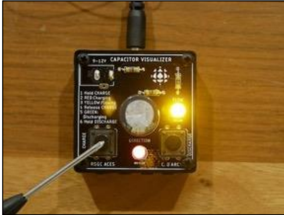
Current flows from positive to negative filling up the capacitor and dimming the red LED (PCB)
