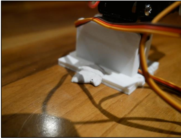
Using sticky tack to hold down th motor case Incorrect angle formula on the case (the bottom formula)
