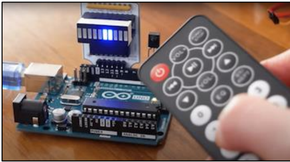
The project setup controlled through IR by a remote
