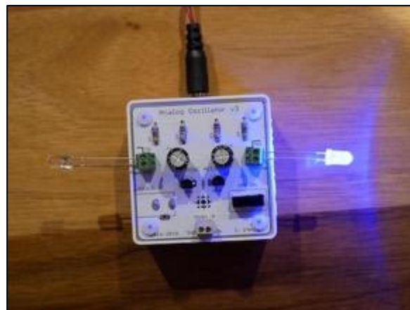
The capacitor charges without the LED, producing non-fading and blinking lights in a square wave
